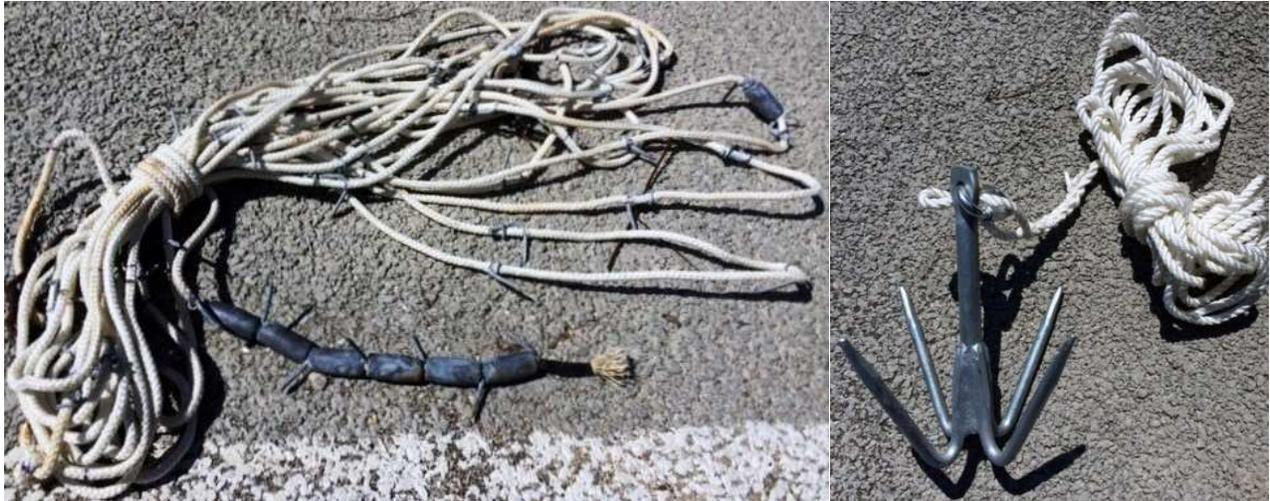
**Figure 3.** Snag line (left) and grappling anchor (right) used to retrieve pots located with side-scan sonar. To construct the snag line, hog rings affixed bent 12-penny nails approximately every six inches. Ends were weighted with approximately four pounds of lead.
