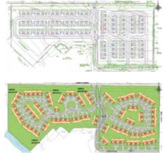
Low-impact development requires looking at development different. Here is a site plan using conventional development techniques (top), which will result in a monotonous, cookie-cutter subdivision that will produce a huge flow of stormwater. The LID concept clusters the houses and creates large swaths of green space that will buffer stormwater.
