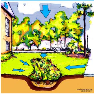
Rain gardens are shallow depressions containing native plants. They work the way nature does. They capture stormwater runoff so it can soak into the ground.
