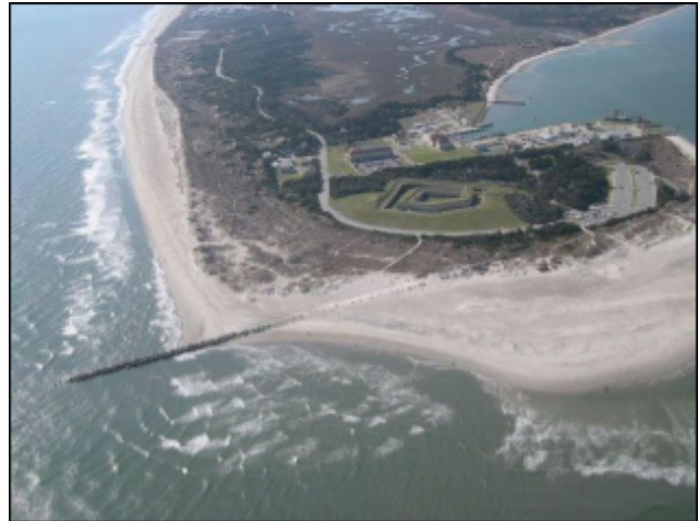
Figure 1. Terminal groin located on the east side of Fort Macon in Carteret County, NC. Photo by Greg Rudolph.
