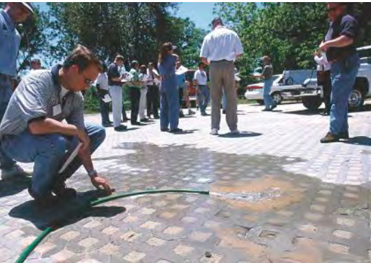
Permeable paving demonstration
