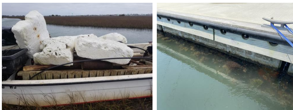
Unencapsulated floats (left) shed polystyrene particles and break apart in the marine environment, as opposed to encapsulated (right) which do not.
