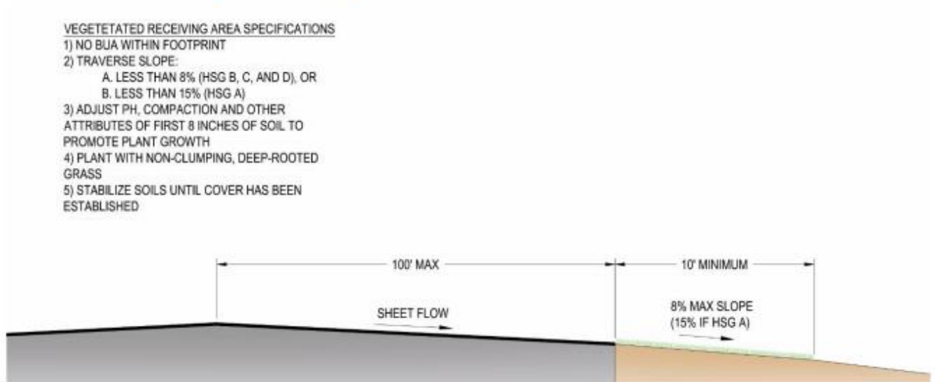
Figure 2: Example Disconnected Pavement: Plan View
