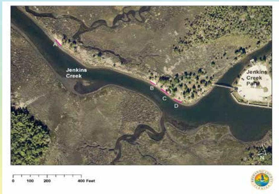
Site description: The site is approximate 50 ft long with 950 SF of barren soil. The land is eroded from runoff with an approximate 2 feet elevation difference.
