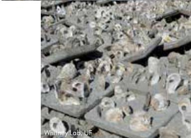
**Community Oyster Reef Enhancement (CORE) modules** are lightweight, easy to produce, plastic-free structures constructed from concrete and an organic mix (wood chips and burlap) with partially embedded recycled oyster shells. Each module contains ten vertically oriented oyster shells, measures 11x14 inches, and weighs about 6-8 pounds.
