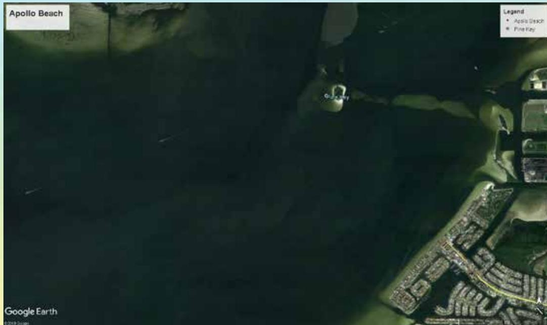
Site description: The site is approximately 800 feet long with severely eroded shoreline due to vast open water fetch conditions, most of this site has a 6-8' escarpment. The land is eroded due to wind driven waves as well as ship wakes.
