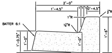
MODIFIED TYPE "A" CURB AND GUTTER
