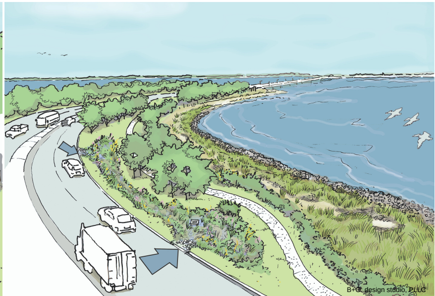
A coastal road uses curb cuts to guide runoff to a roadside infiltration system. Permeable paving on the bike path disconnects runoff and a living shoreline was installed to reduce soundside erosion to protect the roadway.
