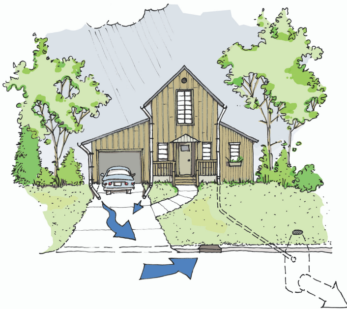
Stormwater runoff flows from this conventional home when rain hits the impervious roof, walkway and driveway. The polluted runoff then flows to the storm drain where it can reach surface waters.
