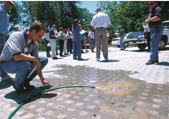
Permeable paving demonstration
