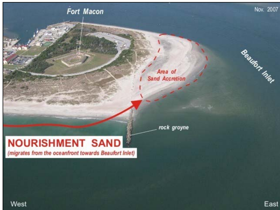
Figure 11. As nourished sand is put on the beach, the sand moves toward the inlet and through the terminal groin to just inside the western edge of Beaufort Inlet.
