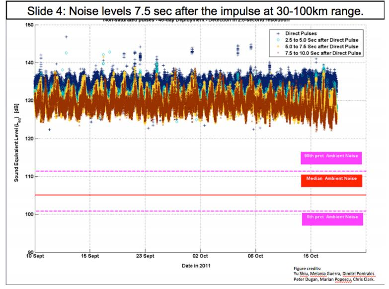
Noise levels at the time of, 2.5-5, 5-7.5 and 7.5-10 seconds after a seismic survey pulse. Note the significantly elevated noise levels even many seconds after the pulse. Ambient noise levels are shown with red and pink lines. It is important to remember that every increase of 10 dB represents an order of magnitude increase in sound intensity; so even between pulses the ambient noise is elevated by 1-2 orders of magnitude. This result is corroborated by published studies (Guerra et al., 2011).
