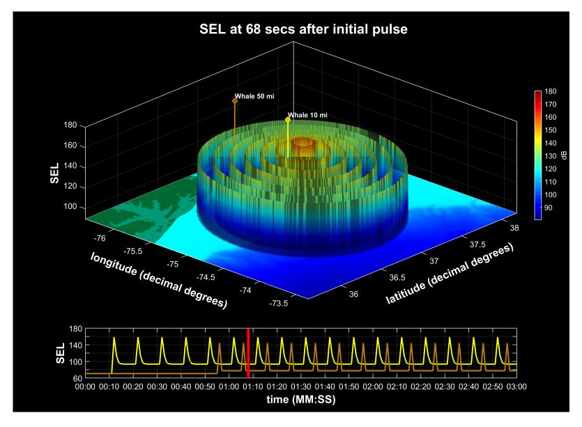
Another perspective on Figure 1. This plot shows the levels (bottom) of sound reaching the two whales in the sound field.
