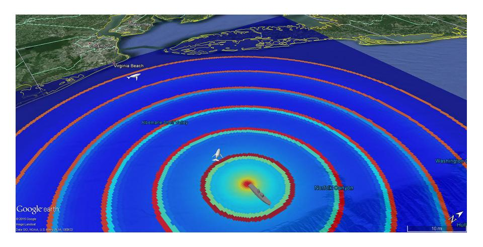
The sound field 60 seconds after the initial seismic survey pulse produced by the vessel near the Norfolk Canyon off the coast of Virginia. The levels experienced by the close whale are almost continuously at or above levels known to impact baleen whales, and the distant whale experiences these levels for the ~10 seconds around the time of the pulse. The dark red color maps to approximately 175 dB, the light green to 125 dB, and the light blue to 100 dB.
