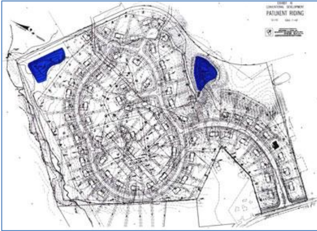
Image 1: Design using conventional “pipe and pond” stormwater management.
