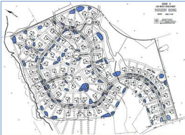
Image 2: Design featuring LID-based stormwater management utilizing smaller integrated stormwater management practices.
